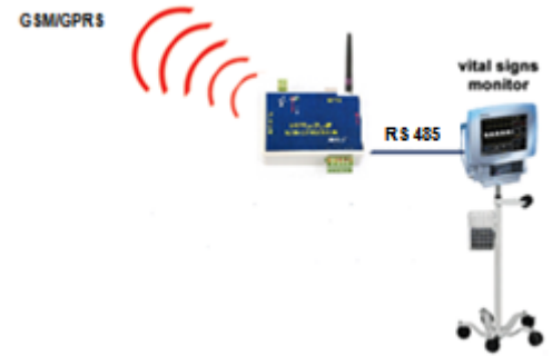
Figure: Wireless Device Server-GSM used in hospitals for monitoring
