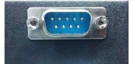
DB 9 Male connector for RS232/RS485
