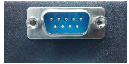
DB 9 Male connector for RS232
